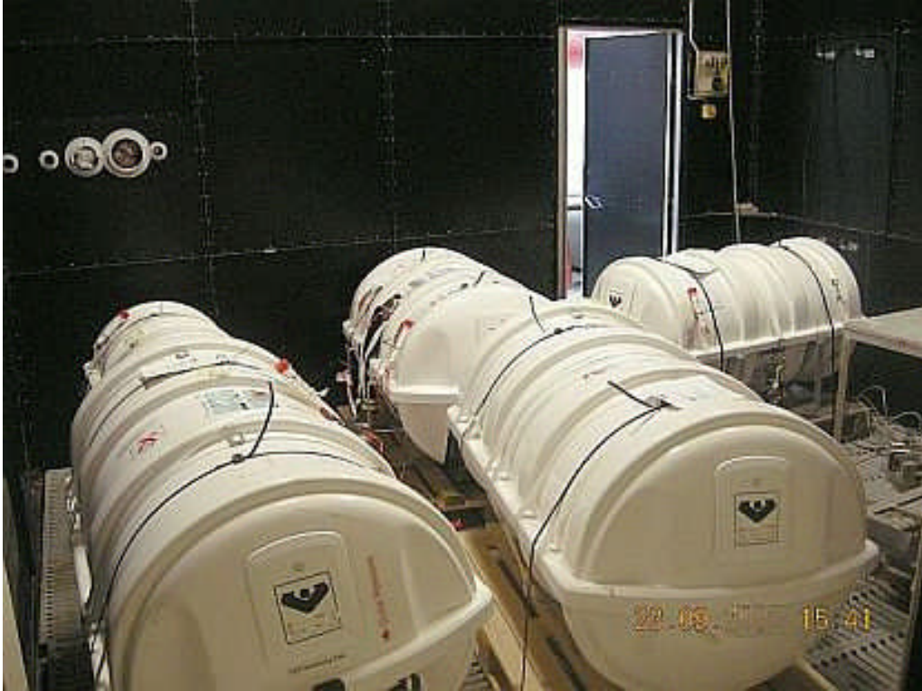
FIG 5.2.1.2 The inside of a larger climatic chamber.
